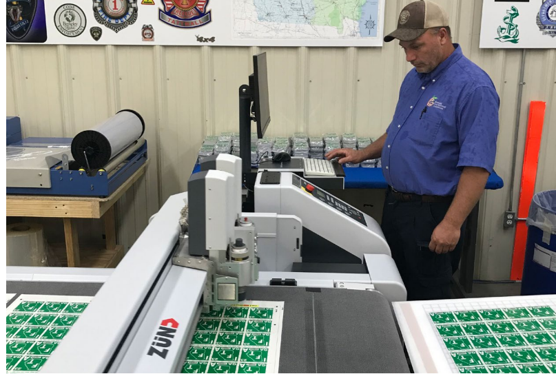
Reading the art file dots and adjusting the camera on the digital flatbed cutter. This will allow for the cutting automation.
