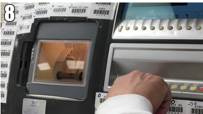
8 Kappa edger cuts lenses using a special cutting wheel
